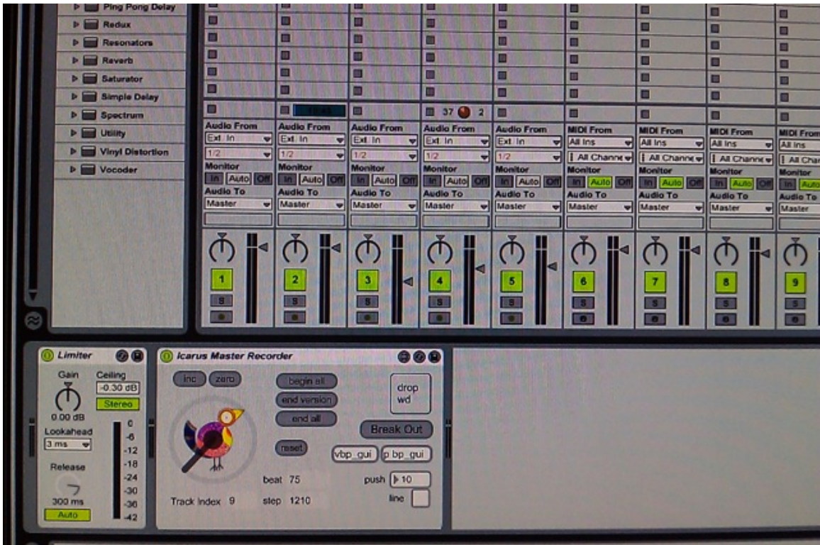
Figure 2: A live project showing the process of interpolation between breakpoint functions (lower two track lanes) to produce a resulting interpolated pattern (upper right breakpoint function). The upper left breakpoint function describes a mapping from the version dial (x-axis) to the actual value used to interpolate between the input breakpoint functions. This could be repeated multiple times for each piece. In the top right the outputted renderings are shown being recorded into a directory.
